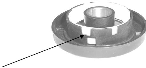
The thin area between the crank position and the cylinder position is the most common breakout location.
