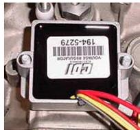
9. Connect all wires to the regulator/rectifier, matching color codes (the gray stripe on the OEM stator can be connected to either yellow wire on the regulator/rectifier).
