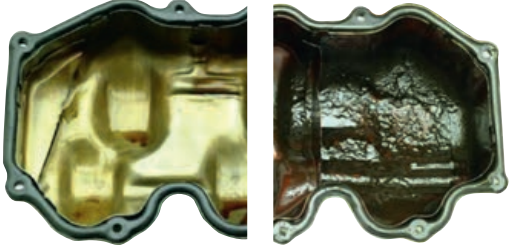
Engine detergency test after 300 hours Neglecting oil changes or using poorer quality oil (right) instead of Yamalube (left) can lead to clear performance differences.
