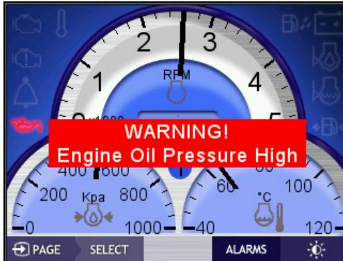
**Figure 46: EGM Performance Alarm and Warning**
